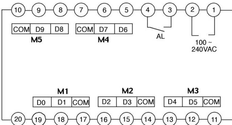
D0-D7 for external alarm switches inputs. D8 is for silencer switch input, and D9 for test switch input. AL is for relay output. ALL the COMs are the common terminals and internal connected.
