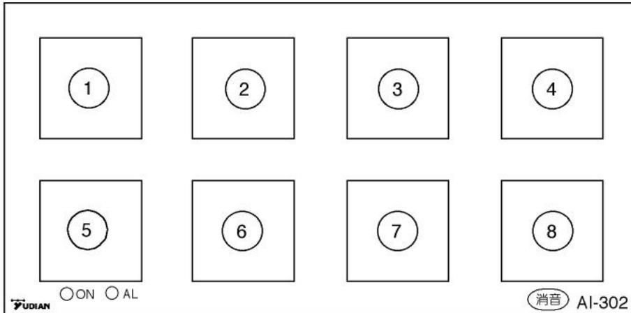
When D0~D7 is connected to COM terminal, the corresponding LED light 1~8 will flashing.
